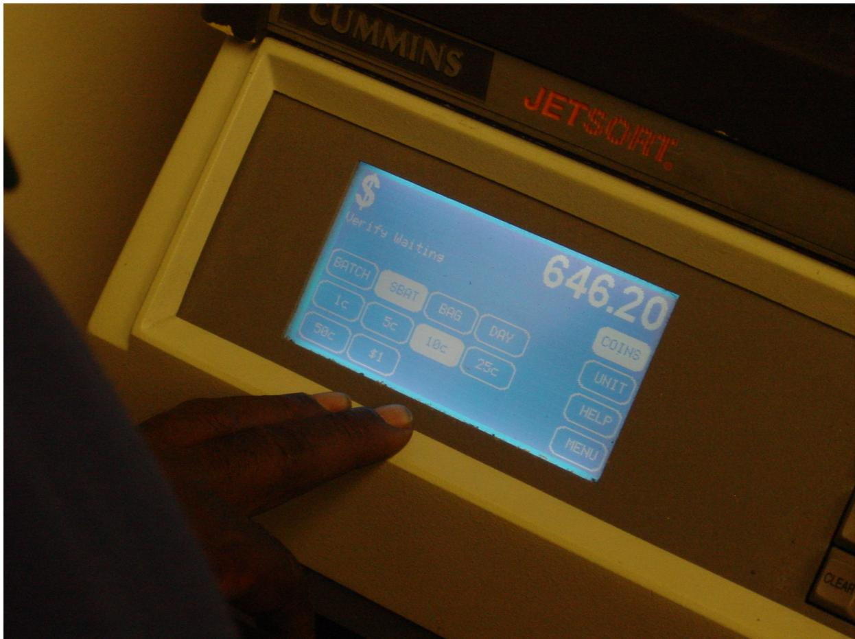
*A typical coin counter deployed in parking and toll count rooms. This is a Cummins Allison Jet Sort model. Photo courtesy of The H2H2H Foundation.*
